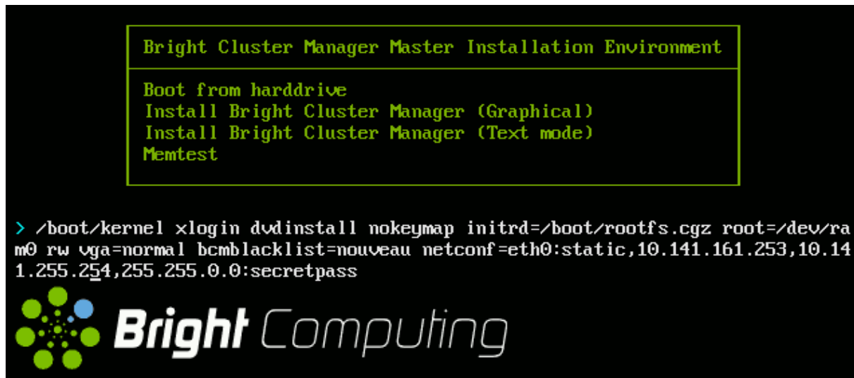
Figure 3.1: Installation: ISO Boot Menu For Legacy BIOS
