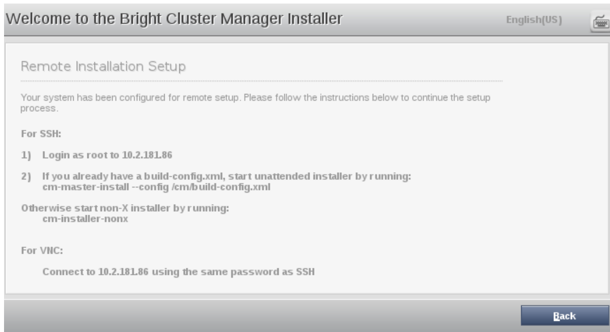
Figure 3.5: Remote Installation: VNC and SSH access explanation
